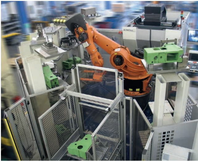
Flexible production cell with pallet station. ALZMETALL is using their proper machining centers.
