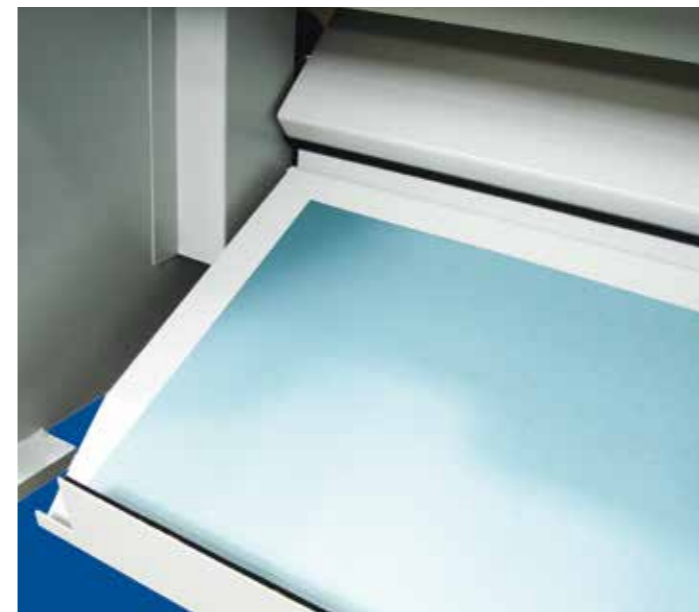
Parts chute for cut piece delivery to the front.
