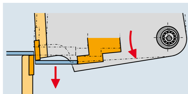
The tilting motion of the swing beam eliminates parts getting stuck between the lower blade and the backgauge.
