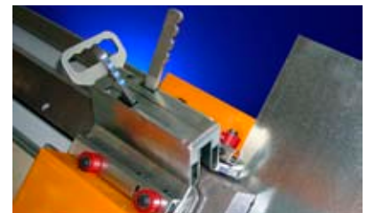
Safe two point sheet clamping
