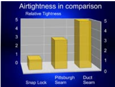
The Duct Seam is much tighter than other common seams such as Pittsburgh or SnapLock
