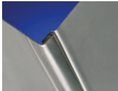
Equipped with specific forming rolls the DuctZipper RAS 20.10 can also handle 0.8 mm (22 Ga.) stainless steel material
