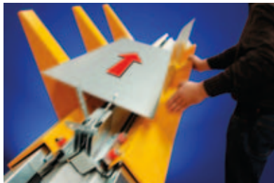
Easy slide-back of semifinished ducts to the entry point
